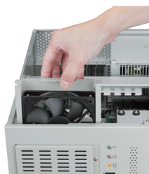
Easy-to-maintain cooling fan
